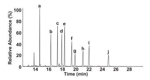
Figure 1. Typical gas chromatograph–mass spectrometer chromatogram with all phytoestrogens. a,  $5\alpha$ -androstane- $3\beta$ ,  $17\beta$ -diol; b, formononetin; c, daidzein; d, genistein; e, secoisolariciresinol; f, coumestrol; g, glycitein; h, matairesinol; i, lariciresinol; j, pinoresinol.
